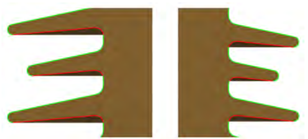
Figure 3: Comparative illustration of shed profiles: LEFT illustration shows old design (generation I design) – porcelain long rod insulators with specific creepage distance of 50 mm/kV. RIGHT illustration shows new design (generation II design) – for unified and optimised porcelain long rod insulators for all specific creepage distances ranging from 31 mm/kV up to 50 mm/kV.
