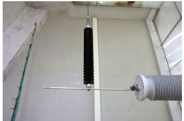
Figure 9: General set-up as test arrangement for all a.c. pollution tests on porcelain long rod insulator (for generation I & generation II) designs with specific creepage distance as 50 mm/kV.
